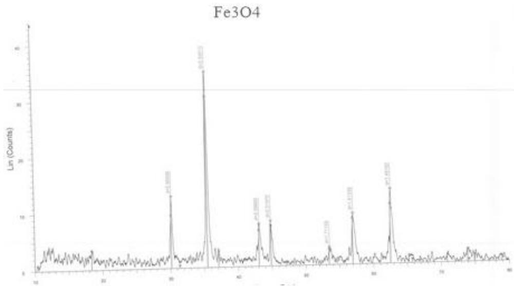
**Fig.2.** XRD pattern of *Fe<sub>3</sub>O<sub>4</sub>* monocrystalline.
