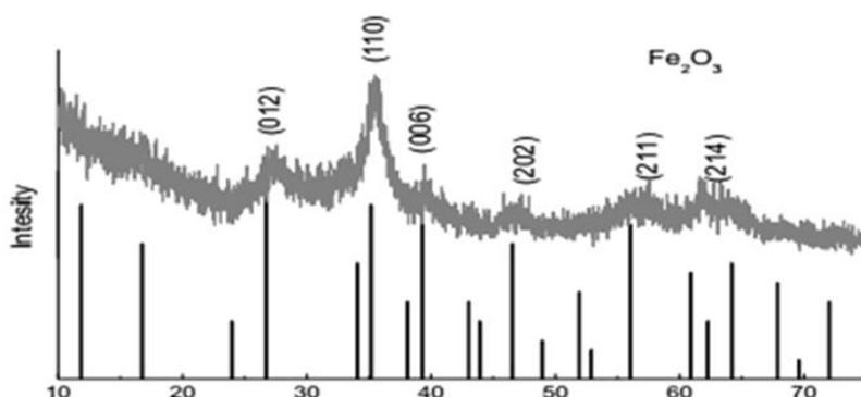
**Fig.1.** XRD pattern of Fe<sub>2</sub>O<sub>3</sub> nanocrystalline sample
