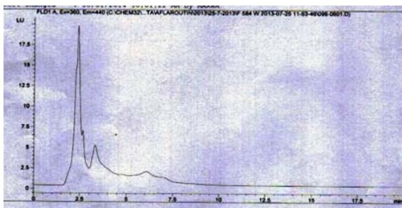
Fig (4) Quantification of aflatoxin in *A.niger* extract by HPLC.
